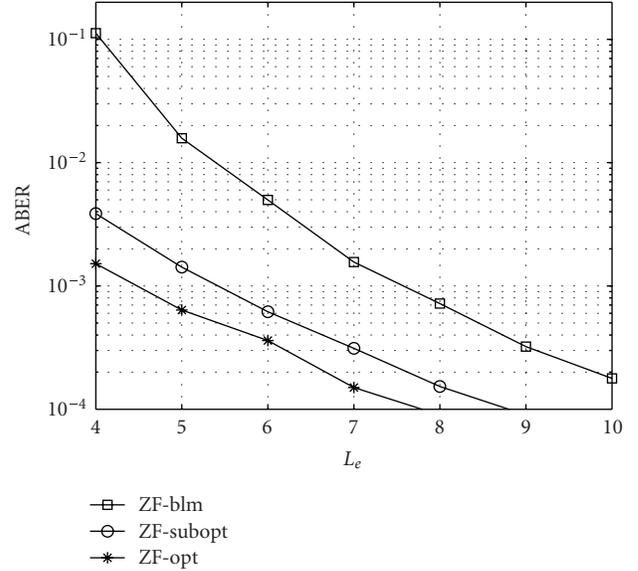
FIGURE 3: ABER versus  $L_e$  ( $T_s = 160 \mu\text{s}$ ,  $f_{\max} = 100 \text{ Hz}$ ,  $N = 2$ ,  $Q_e = 18$ , and  $\text{SNR} = 20 \text{ dB}$ ).
