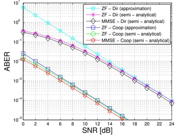
Fig. 7. ABER versus the SNR for  $N_C = 6$  relays in the case of the  $(N_S, N_R, N_D) = (2, 2, 3)$  antenna configuration (Example 2).
