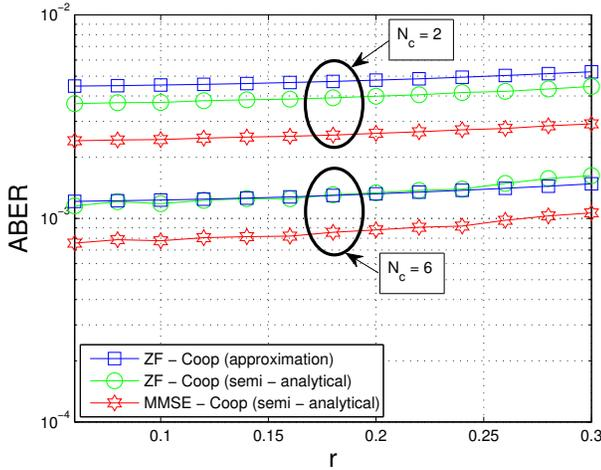
Fig. 3. ABER versus the cluster's radius  $r$  for two different values of the number  $N_C \in \{2, 6\}$  of relays (Example 1).
