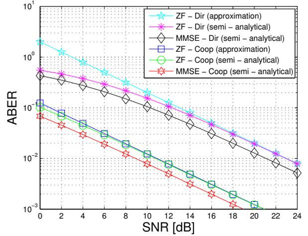
Fig. 5. ABER versus the SNR for  $N_C = 6$  relays in the case of the  $(N_S, N_R, N_D) = (2, 2, 2)$  antenna configuration (Example 2).
