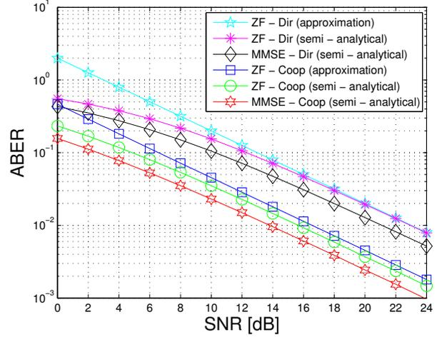
Fig. 4. ABER versus the SNR for  $N_C = 2$  relays in the case of the  $(N_S, N_R, N_D) = (2, 2, 2)$  antenna configuration (Example 2).
