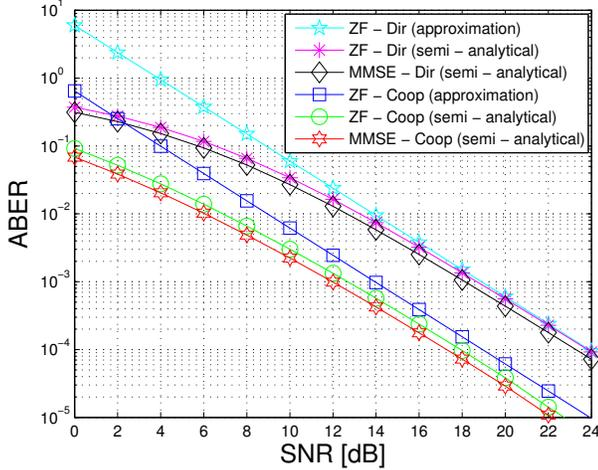
Fig. 6. ABER versus the SNR for  $N_C = 2$  relays in the case of the  $(N_S, N_R, N_D) = (2, 2, 3)$  antenna configuration (Example 2).
